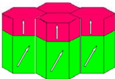
Soft material with volume  $V_{soft}$ . Facilitate switching of the grain.
