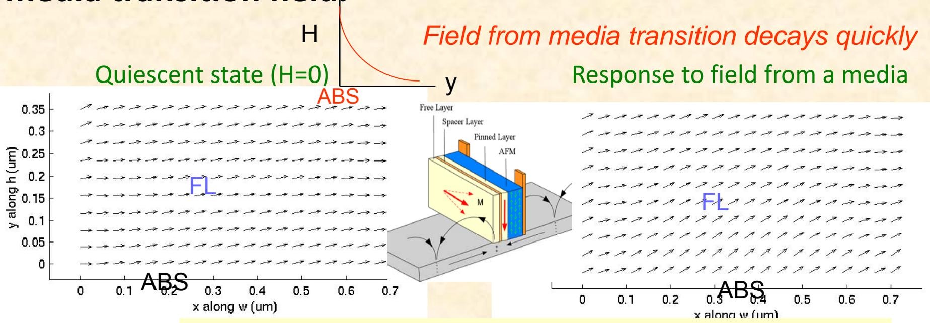
**Shape anisotropy limits response for smaller devices.**
