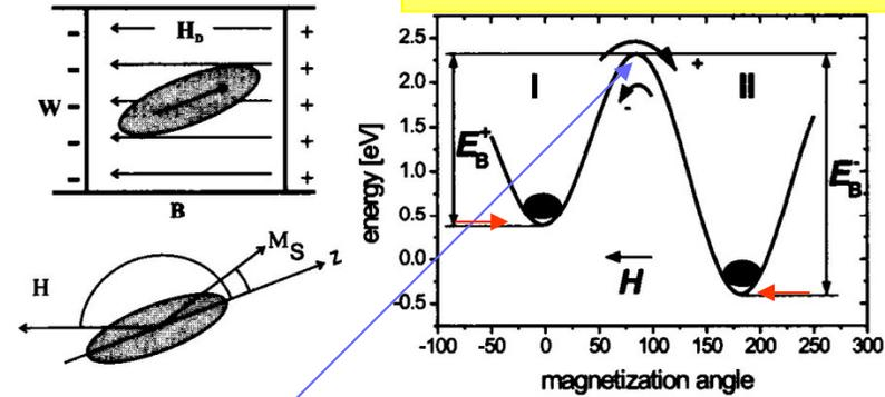
$\Delta E = (\text{crystal anisotropy})(\text{grain volume}) = K \cdot V$
