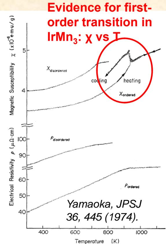
Fig. 5. Temperature dependences of magnetic susceptibility  $\chi$  and electrical resistivity  $\rho$  of the partially ordered ( $S=0.83$ ) alloy compared with those of the disordered ( $S<0.08$ ) alloy with  $x=0.256$ . Open circles indicate the cooling process.
