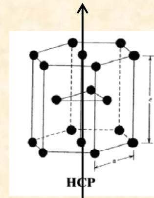
Anisotropy axis out of plane
