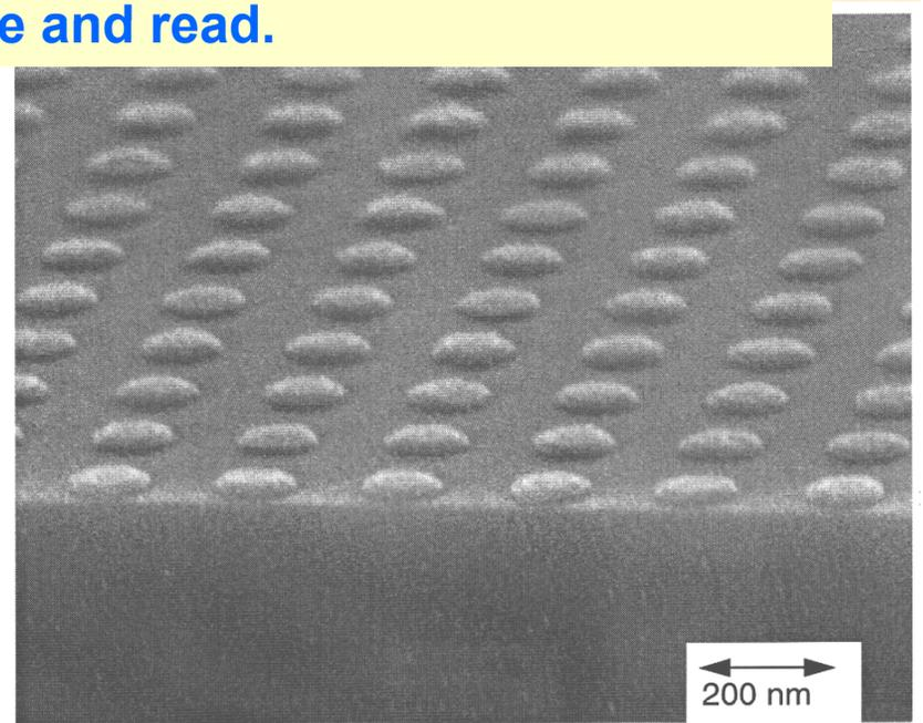
100 nm diameter Co/Cu bilayer dots with 200 nm period
