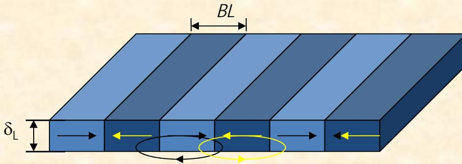
Magnetostatic fields destabilize the transitions (superparamagnetism).
