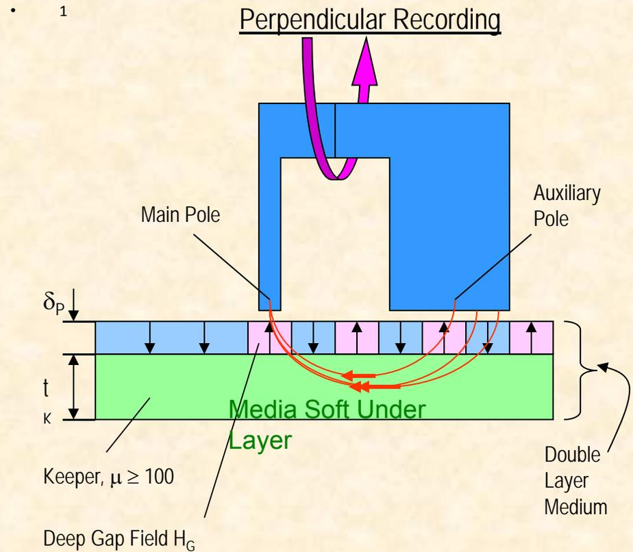
Double layer perpendicular media with soft magnetic Underlayer: media becomes part of the write element
